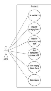
The front end needs to exhibit in full detail and with great scalability all the content required by the EV operator, whether for a simple conference or a deeper analysis. For instance, Figure 4 shows the use case diagram for the front-end service.
